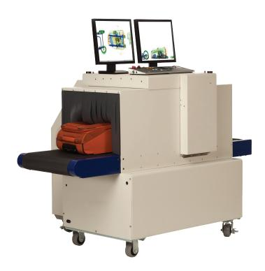
The 6040-DV multi-energy X-ray scanner delivers a clear picture of hidden explosives, weapons, drugs and other contraband in hand-carried and small-to mid-sized items. This dual-view system displays two separate, perpendicular X-ray images to provide a complete inspection in a single scan. Our autoSoft operating system gives a bold boost to our suite of image enhancement tools, allowing operators to more quickly and easily manipulate image data for the best possible picture of concealed threats.
